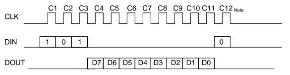
The DIN data in C1~C3 cycle is R08 command, C1 is MSB, C3 is LSB. The DOUT data in C4~C11 cycles are the output data from Register 08, D7 =  $R08_7$ , D6 =  $R08_6$ ,.....D0 =  $R08_0$ .
